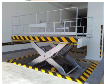
Scissor lift (Lever, screw, rack gear)
