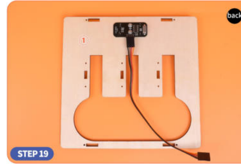
● Install the ultrasonic module on the back of board 1 using a 4mm coarse-thread screw.
