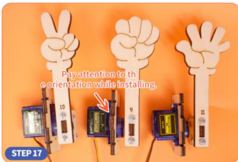
● Refer to the installation method shown in STEP 16 to install the remaining two servo horns from board 6 onto the servo motors.
