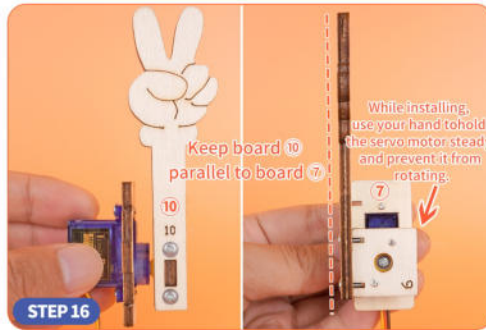
● Install the servo horn on the servo motor of board 6 using a 7mm coarse-threaded screw. Note: Hold the servo motor steady with your hand while installing and ensure it does not rotate.
