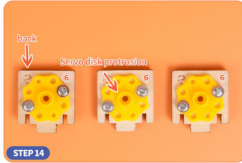
● Install the three steering gear discs on the back of the three No. 6.
