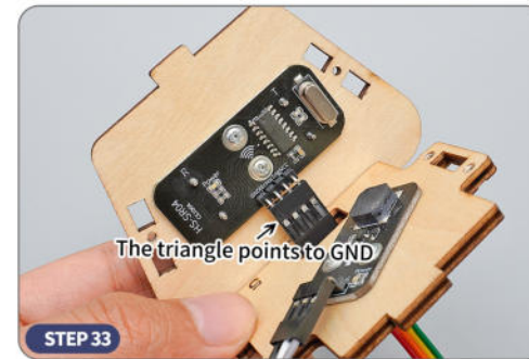
STEP 33 ● Plug a 4P DuPont cable port through the cable hole in board (5) to the ultrasonic module connector.
