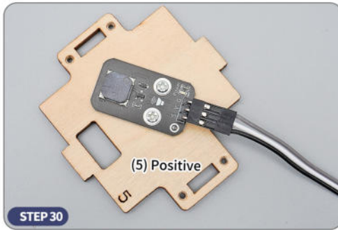
STEP 30 ● Install the passive buzzer on board (5) with 4mm rough screws.
