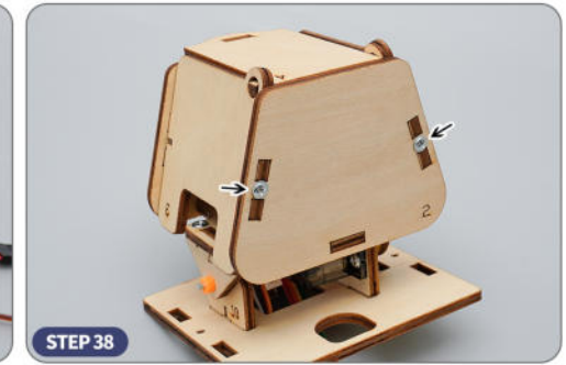
STEP 38 ● First install the (2) plate on two (3) and (5) plates, and then fix it with 7mm rough screws.
