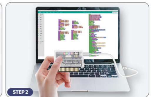
● Use the Mixly software to upload the kit's initializer to the U+ program card.
