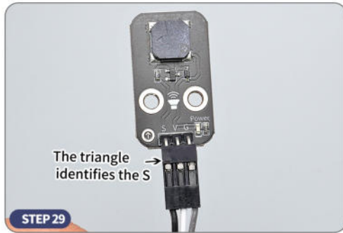
STEP 29 ● Plug a 3P DuPont cable port into the passive buzzer connector.
