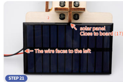
STEP 21 Refer to the picture above, glue the solar panel to board (2) with the wire facing to the left.
