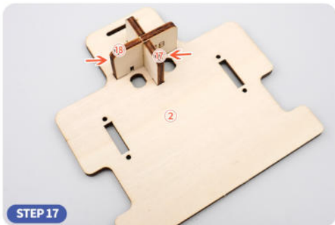
STEP 17 Referring to the figure above, first align the (17) board and install it on the (2) board, and then snap the (18) board into the (17) board and install it on the (2) board.
