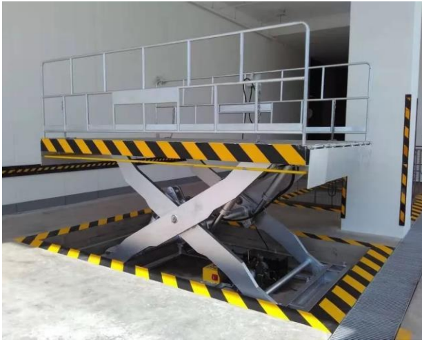
Figure 9 Scissor lift (Lever, screw, toothed bar)
