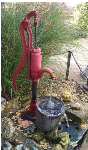
Figure 6 Manual water pump (Lever and axle)
