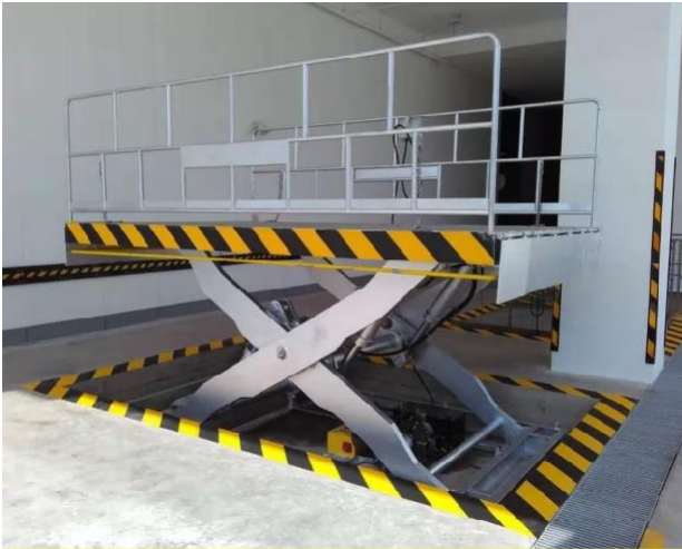
Figure 9 Scissor lift (Lever, screw, toothed bar)
