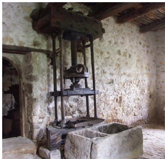
Figure 7 Olive press (Lever, screw & axle)
